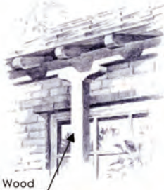
Corbeled Wood Columns
