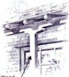
Corbeled Wood Columns
