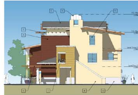
1 BLDG. 4 - East Elevation (BLDG. 5 - West Sim) Scale: 1/8" = 1'-0"
