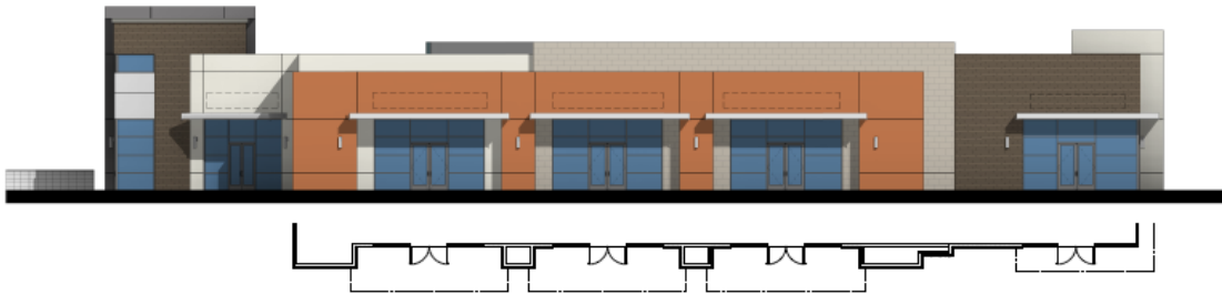
③ BLDG B SOUTH ELEVATION 1/8" = 1'-0"
