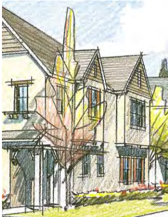
Cantilevered second floor pop-outs with siding accents at gable ends.
