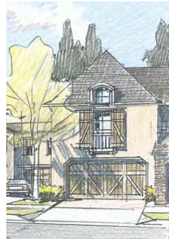
Windows are placed in alignment. Garage door is enhanced and recessed with shadow line even though it is located forward in plan.
