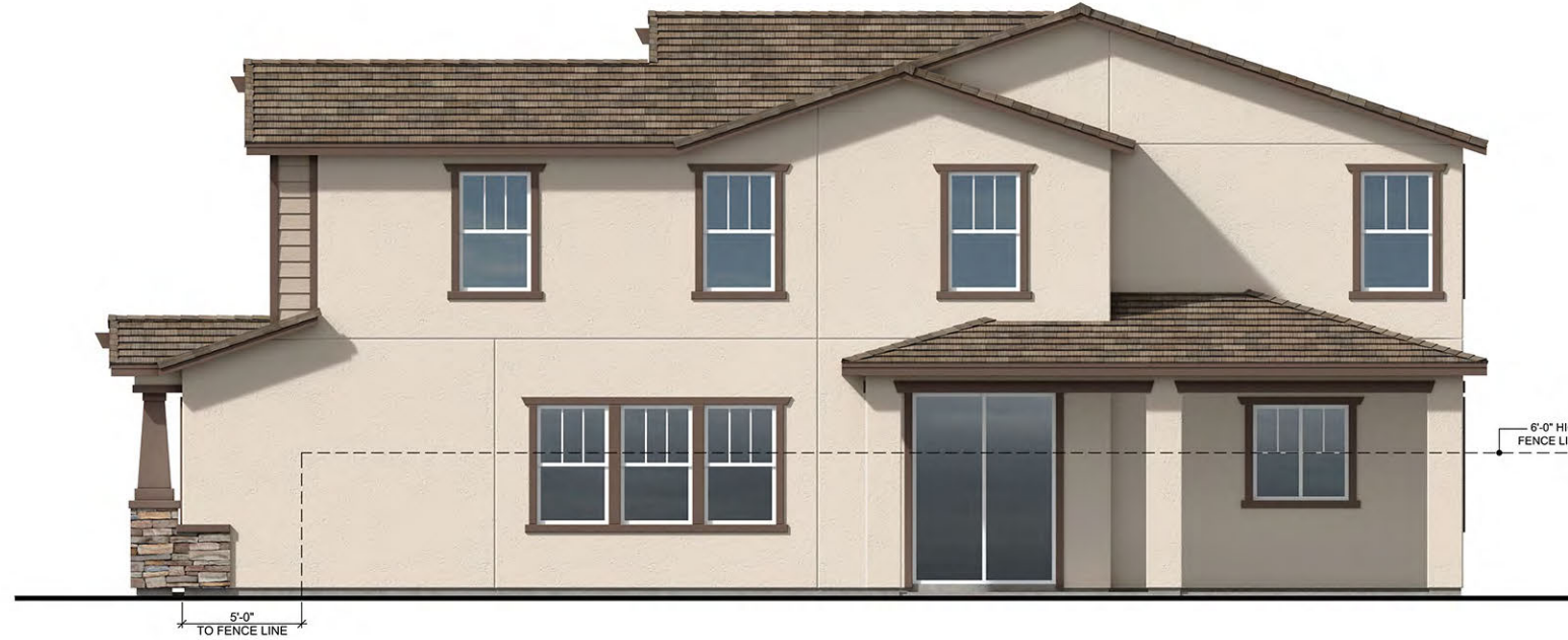
Right Elevation 'B' (Craftsman) at Covered Patio
