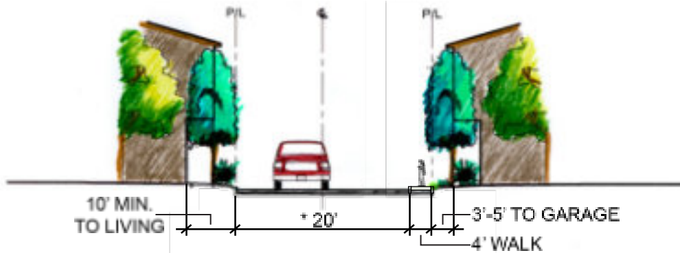
Exhibit 17m-2 - Private Drive (Cross-Section and Plan)
