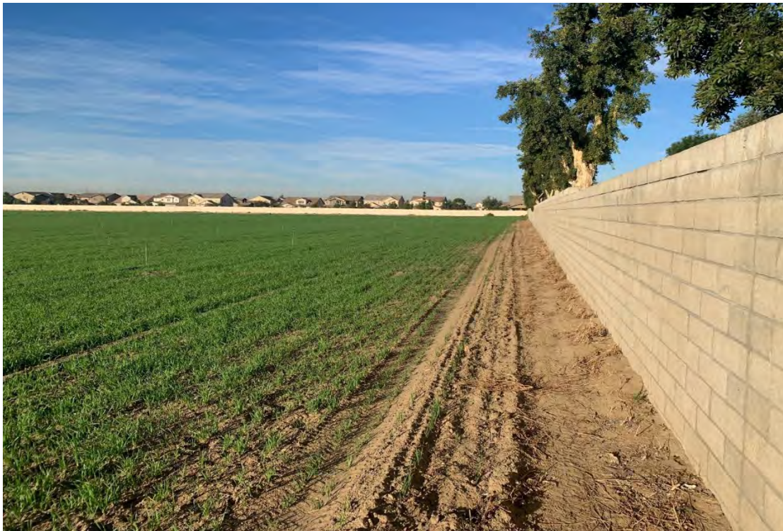
Photograph 6. Looking North from the center of the site, along the north boundary. Note the dark color and clumping of the soils, indicative of the high clay content of the soils.
