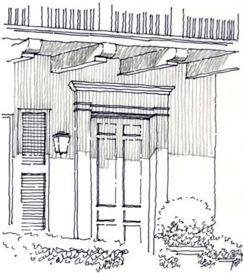
Protected Door Under Balcony
