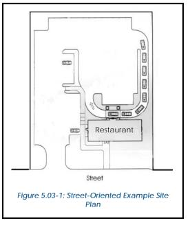
thoroughfare, but instead shall take access from a parking area or on-site drive aisle, as exemplified by Figure 5.03-1 (Street-Oriented Example Site Plan).
