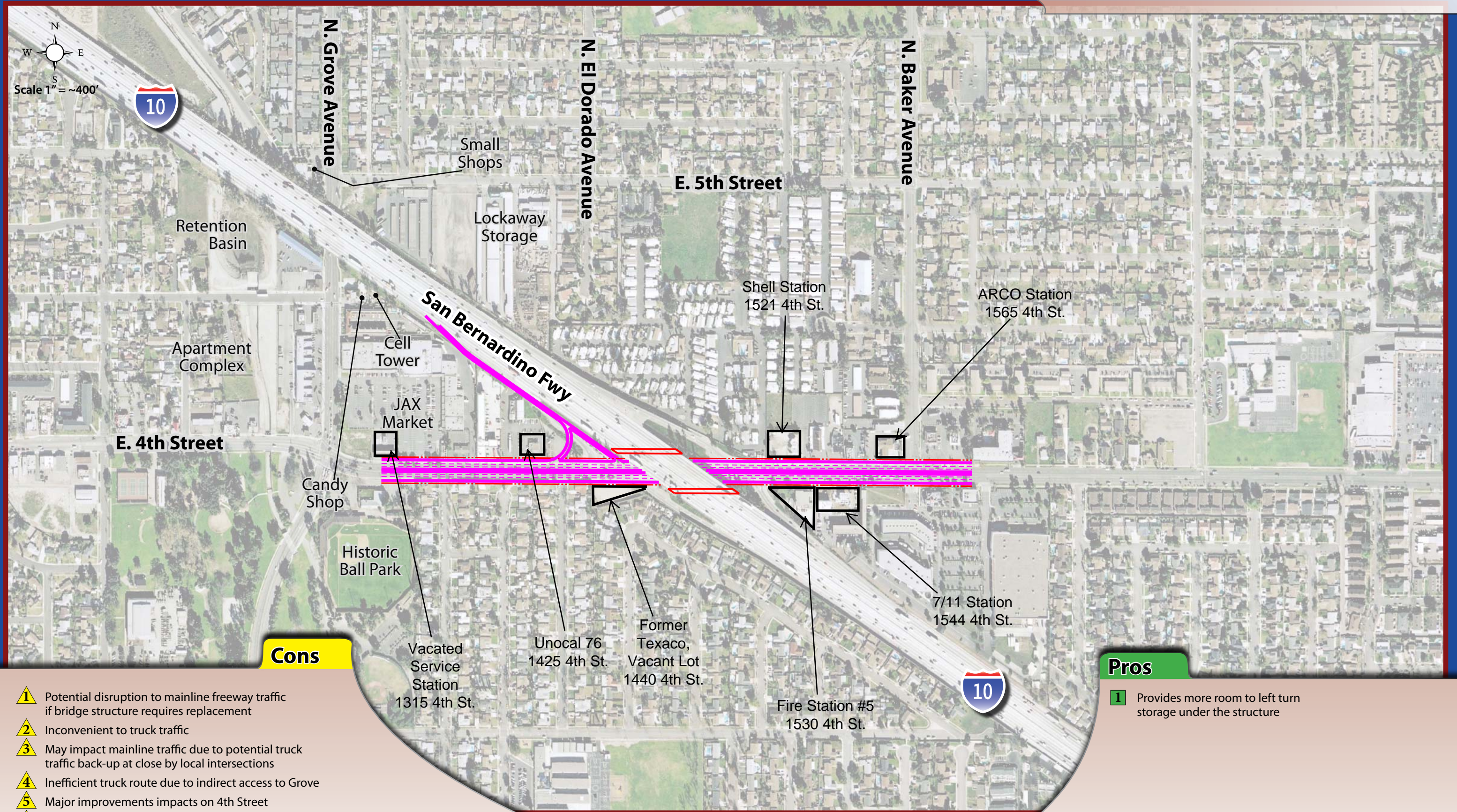
FIGURE 8 Interchange Alternative 6 Bridge widening of 4th street
