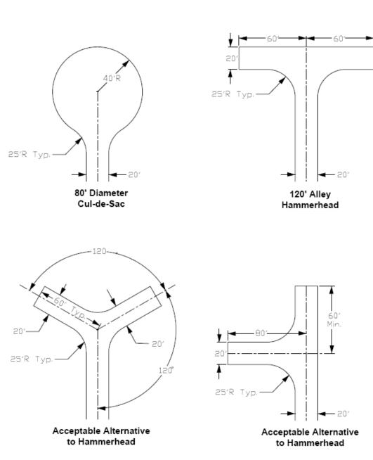
Acceptable turnarounds for all fire access roadways greater than 150' in length when non-circulating access is permitted.
