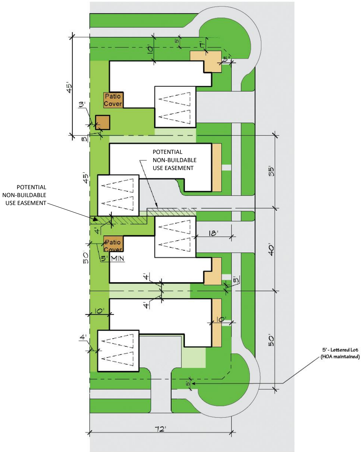
TWO-PACK OR "Z" LOT SINGLE FAMILY DETACHED *Building footprints are conceptual. Actual floor plans may differ.
