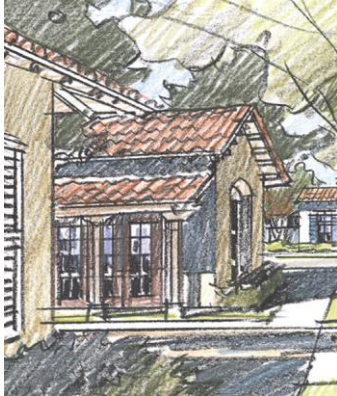
Simple roof forms with exposed rafter tails, porch with shed roof.
