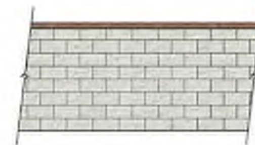
COMMUNITY THEME WALL Community theme colored split-face block wall along project border.
