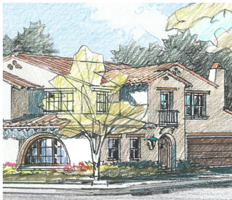
Low pitched gabled roof forms with simple pipe detailing at gable ends.
