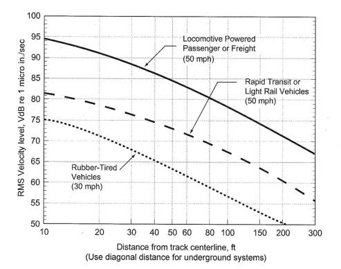
Internal attenuation would reduce the vibration level by an additional 3 VdB. The interior vibration level at the closest possible future home or office would be as follows (VdB):
