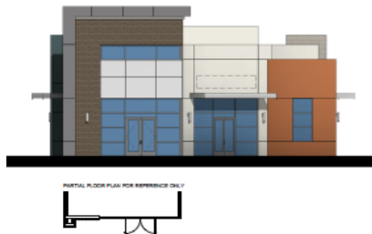
② BLDG B WEST ELEVATION 1/8" = 1'-0"
