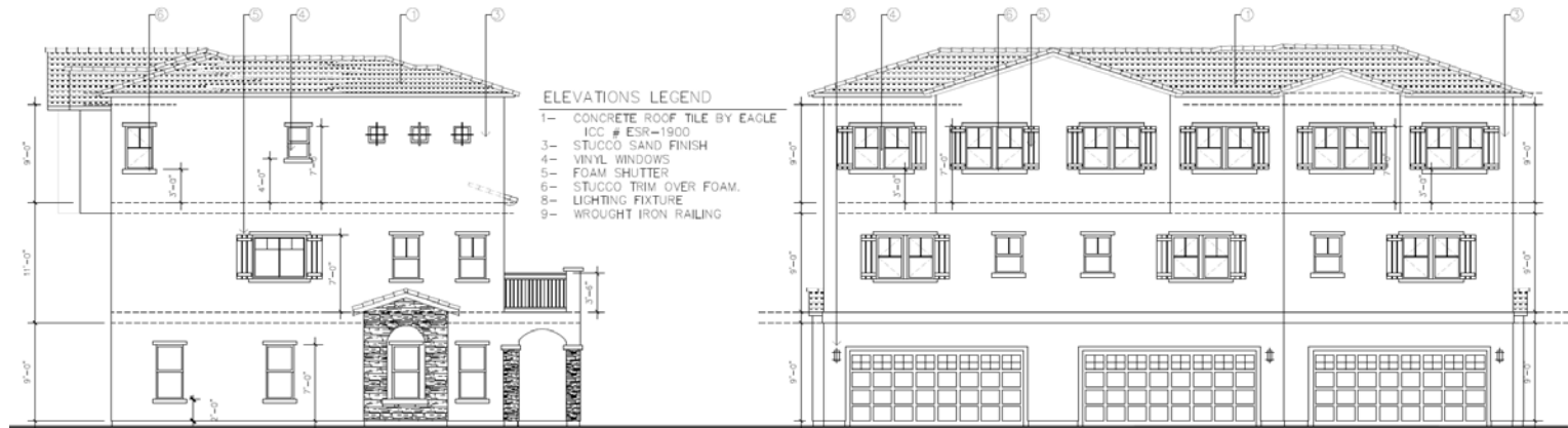
BLDG # 7 NORTH ELEVATION \frac{3}{16}'' = 1'-0''
